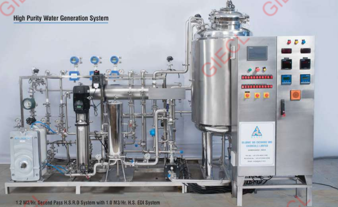
1.2 M3/Hr. Second Pass H.S.R.O System with 1.0 M3/Hr. H.S. EDI System
