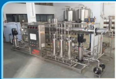
3.0 M3/Hr. Two Pass R.O System with Ultra Pure water production for Pharmaceutical factory
