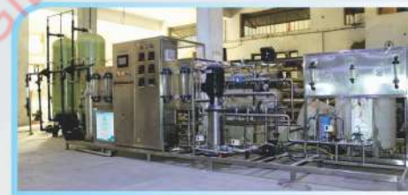
2.0 M3/Hr. Pure Water Generation System for WFI Standard in Pharma industries
