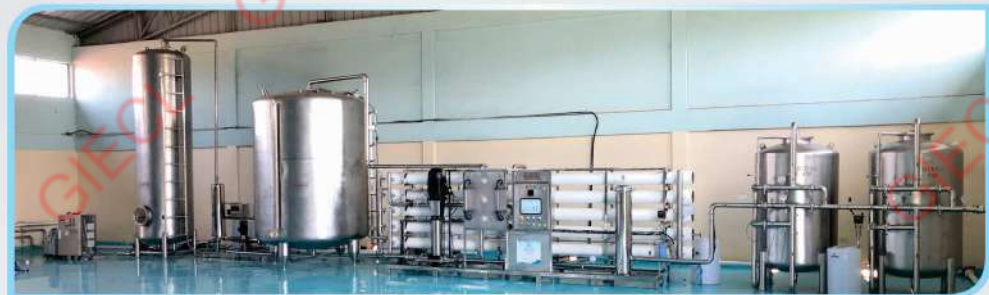
20,000 LPH S.S 316 Mineral Water Plant with Online Mineral Adding System for High Purity Bottled Water
